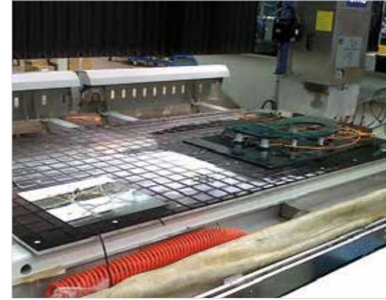
Fully rubberized suction work surface.
