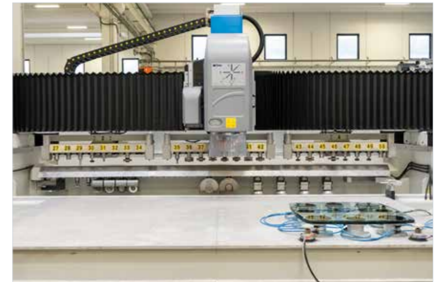
Under-beam tool holder with up to 24 cone positions.
