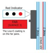
The RED light indicates that a LOW-Ecoating exists on a FAR surface of the window. The far surfaces of the window are surface #3 or #4 as you look at the window.
