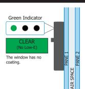
The GREEN light indicates that the window is CLEAR of any LOW-E COATING. NO LOW-E coating exists on any of the surfaces
