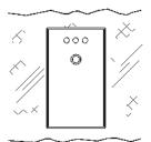
If the window area under test is excessively dirty or contaminated, the ETEKT+ may give improper results. The window area under test must be RELATIVELY CLEAN. Clean the test area or move the ETEKT+ to a clean location on the window.
