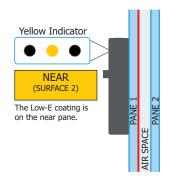
The YELLOW light indicates that a LOW-E coating exists on the NEAR surface of the window. The near surface of the window is surface #2 as you look at the window.
